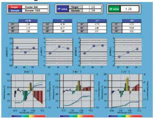
By using the Color Data Software CM-S100w (optional), you can display the data for the 3 different illumination angles simultaneously. Or, you can create a line graph that visually shows the angle characteristics specific to a multi-angle spectrophotometer.
